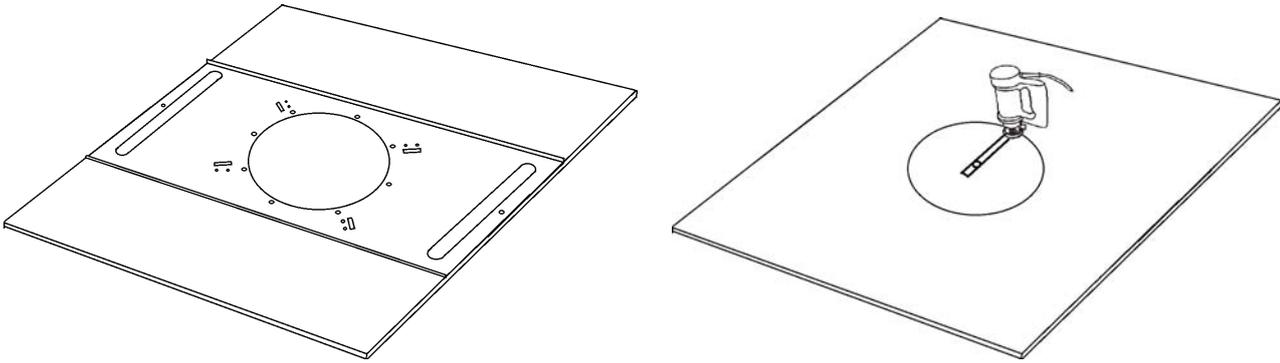
Place the marked tile onto an empty open box or trashcan, to catch any debris. Please make sure to have appropriate clearance for the saw blade and cut the hole with a “plunge’ hand or power saw.
