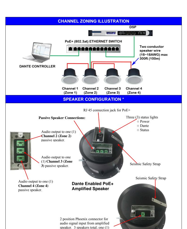
speaker for channel 1 audio and two (2) speakers for channel 2 audio.
