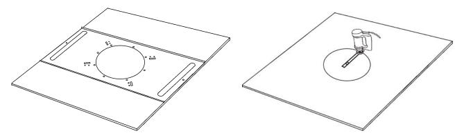
Place the marked tile onto an empty open box or trashcan, to catch any debris. Please make sure to have appropriate clearance for the saw blade and cut the hole with a "plunge' hand or power saw.
