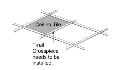
3. Install the T-rail in a rectangular tile – When the ceiling uses rectangular tiles, install the T-rail crosspiece into the ceiling opening up against he cut tile.
