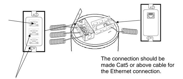
The bottom two connections are for audio output to two (2) passive speakers for different zone (**Channel 2**)
