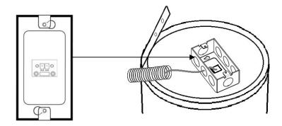
There is a single 2 position phoenix connection inside of the handy box. THE PASSIVE SPEAKER THAT WILL BE THE SAME CHANNEL SPEAKER AS THE ACTIVE SPEAKER HAS **PINK** MARK ON THE PHOENIX CONNECTOR.
