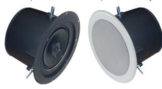
The **AMK PSA802-CFM-4** powered speakers feature a 30 watt Class D digital design amplifier, with > 75% efficiency for the main speaker. These units are available as single master speakers or sets with an unpowered companion speaker (**PSA802-CFM-4-P**) The speaker combines high performance, power handling, and a very smooth response.
