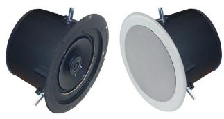
The **AMK PSA802-RPM** powered speakers feature a 30 watt Class D digital design amplifier, with > 75% efficiency for the main speaker. These units are available as single master speakers or sets with an unpowered companion speaker (**PSA802-RPM-P**) The speaker combines high performance, power handling, and a very smooth response.
