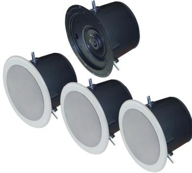
The **AMK QSA615-CFM-2-RVC** self amplified speakers feature a 30 watt class D digital amplifier, with > 75% efficiency for the main speaker. This unit is a quatro system of 4 speakers, one powered speaker and three companion speakers. The speaker combines high performance, power handling, and a very smooth response.
